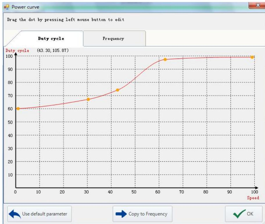
The power curve is fitted as a spline curve, with the horizontal coordinate being the speed and the vertical coordinate being the laser output, which has good smoothness. The interfaces for editing can be chosen as shown above.
