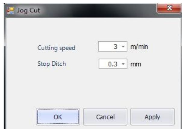
Cutting speed: when the set processing speed is faster than it, it will be the maximum speed limit for jog cutting.
